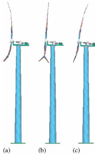
Fig. 5. First flap modes of the wind rotor: (a) collective flap mode, (b) and (c) differential flap modes.
