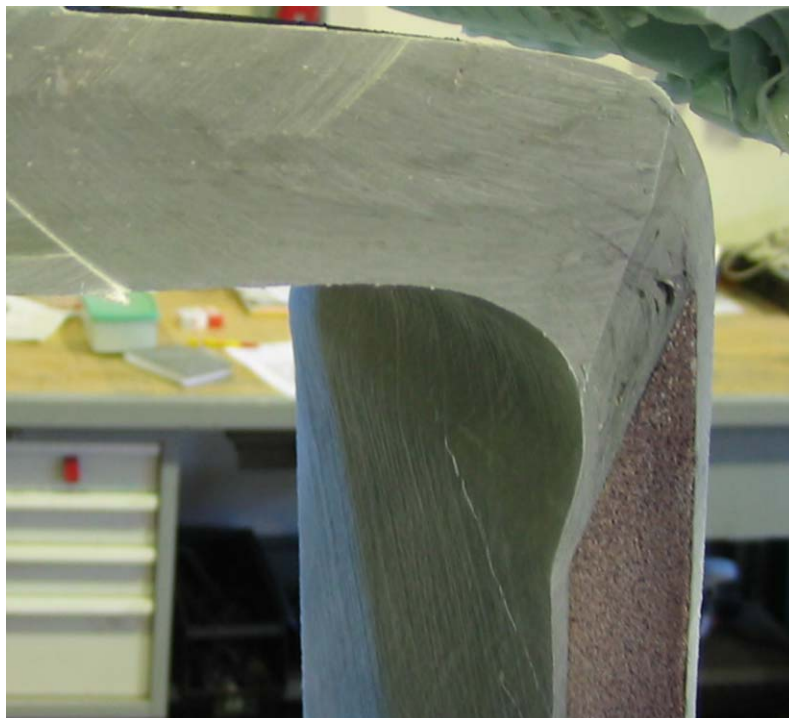
Fig. 14a. Section through a box corner.
