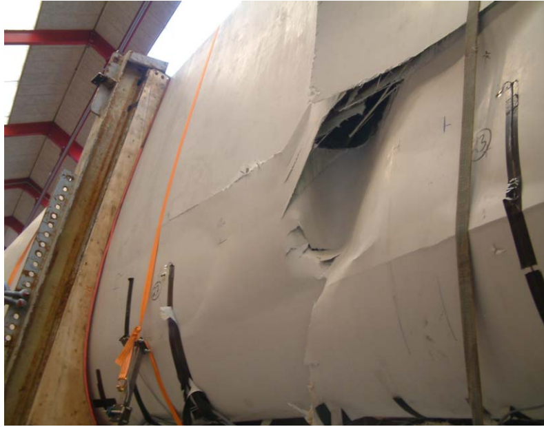
Fig. 9. Buckling collapse.
