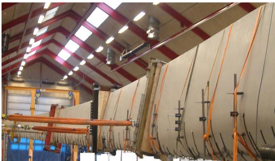
Fig. 1. Full-scale test – flap-wise loading.
