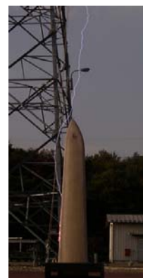
(1)Creeping discharge along trailing edge
