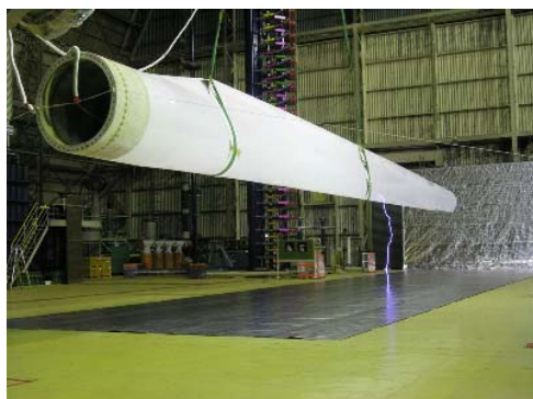
Fig.5. High voltage experiment for real blade
