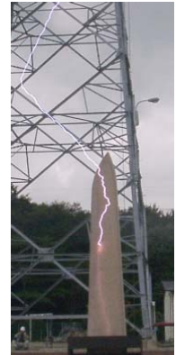
(2)Penetration discharge into the blade
