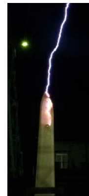
(b)Discharge manner to small disk receptor
