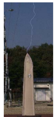
(c)Discharge manner to large disk receptor
