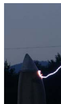
(a)Discharge manner to blade shape receptor
