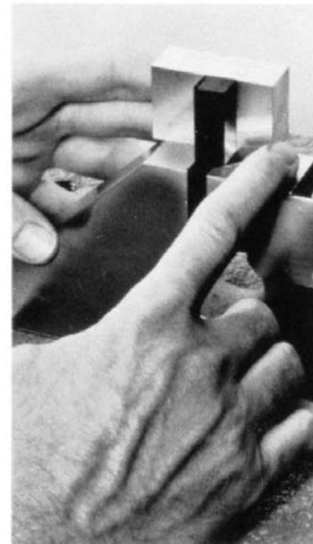
FIG. 4 Jig for Positioning Specimen for Clamping
