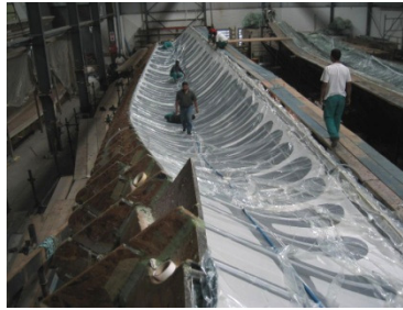
Infusion of a 100' sailing yacht deck and hull by Southernwind Shipyard, Cape Town, South-Africa.
