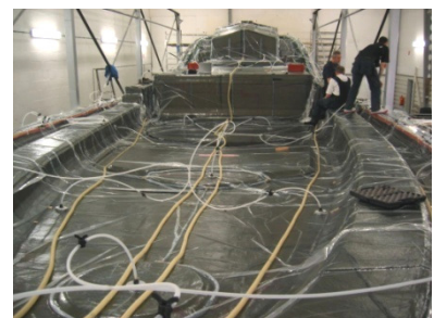
Hull and deck of a 76' high speed powerboat (55+ knots) infused by Pantera Yachts, Waalwijk, the Netherlands.
