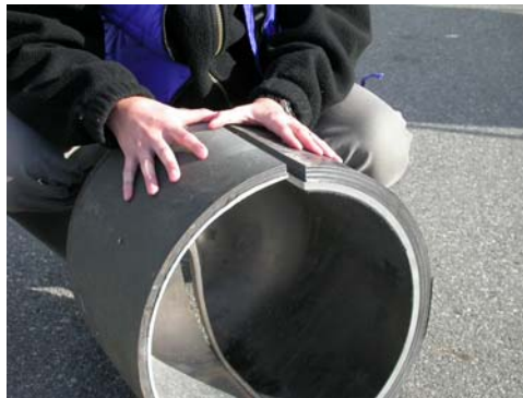
Figure 4: Comparison of wall thickness between a 200 bar and a 700 bar rated Type 3 composite cylinders
