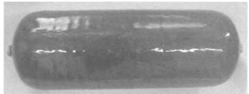
图 4 加工完成的储氢气瓶 Fig. 4 Fabricating completed hydrogen cylinder used as fatigue test object
